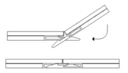
If the panels are not square, or if the edges are not touching along the full length, the panel being fitted will not lower. DO NOT FORCE PANELS DOWN – Simply adjust until it lowers.
