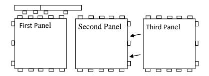
Continue to lay the row with as many full panels as required for the size of the floor, all with the 3 end lugs pointing right.
